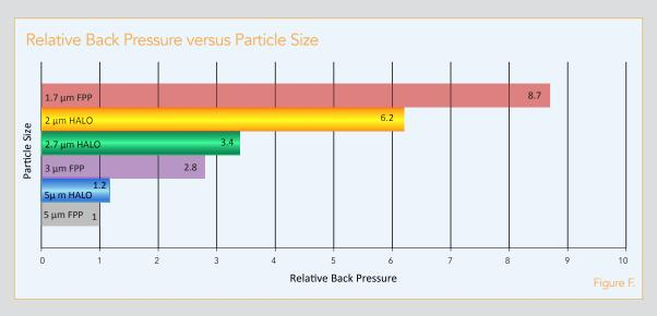
**Example 1:** A 100 mm HALO® column packed with 2.7 µm particles will generate approximately 1.36 times the back pressure of a 250 mm conventional column packed with 5 µm particles.
