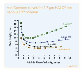
The original HALO® Fused-Core® columns are able to perform competitively versus sub-2 µm fully porous columns and substantially outperform 3 and 5 µm fully porous columns delivering the goal of increased performance without the consequence of high back pressures!
