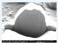
FIB - SEM image of first commercial HALO® particle with 2.7 µm total size consisting of a 1.7 µm solid silica core and a 0.5 µm shell.
