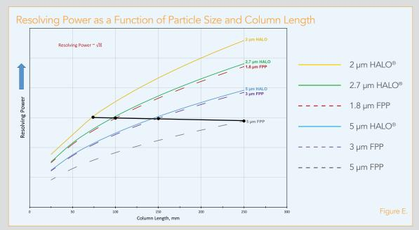
**Example 1:** A 100 mm column packed with 2.7 µm HALO® particles meets the criteria of providing equal or better resolving power compared to a 250 mm column packed with 5 µm FPP particles. The HALO® column is an appropriate choice for replacing the 250 mm length FPP column in an ultra-fast method.
