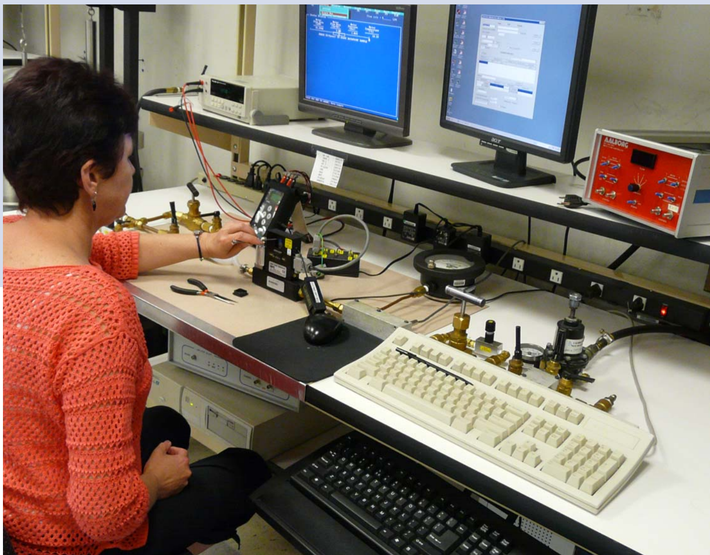
Terminal shown for low-flow Flow Controller calibration supported by Aalborg SDPROC software.
