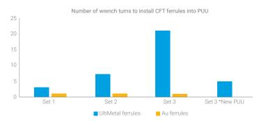
\*Column broke after 20 additional small wrench turns and therefore a new purged ultimate union (PUU) had to be installed.
