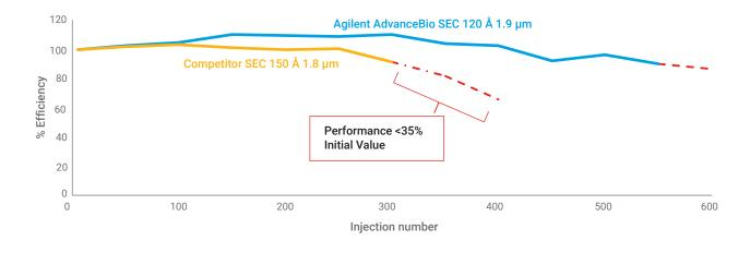
AdvanceBio SEC 120 Å 1.9  $\mu m$  columns showed less than 10% drop in uridine plate number over 550 injections, confirming excellent mechanical stability.
