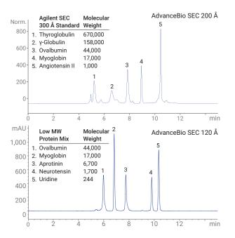
To monitor column and instrument performance, Agilent recommends running a standard test mixture regularly, such as the AdvanceBio SEC standards.
