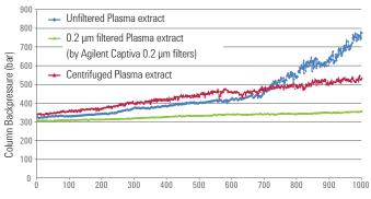
Number of injections of unfiltered, centrifuged, and filtered human plasma PPT Extract.
