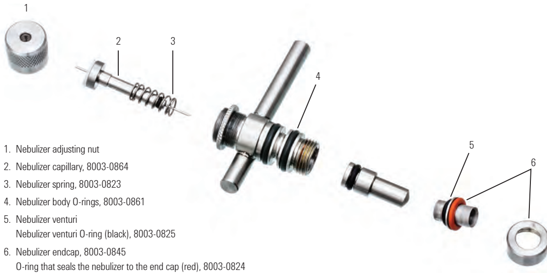
Exploded view of Nebulizer assembly, 8003-0828
