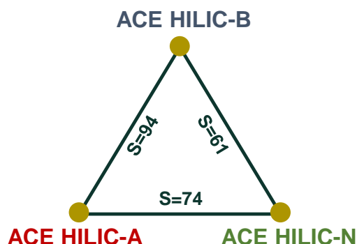
Figure 2 Selectivity triangle for the ACE HILIC range using HILIC probes on 10 mM ammonium formate pH 4.7 MeCN/H 2 O (90:10 v/v)
