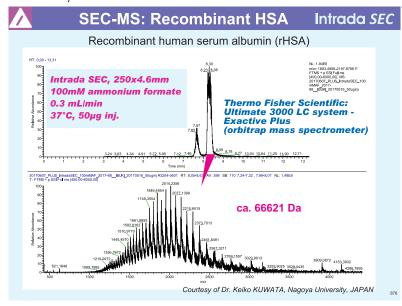
Intrada SEC may be the best SEC column for use on MS detectors, due to its use of volatile eluents.
