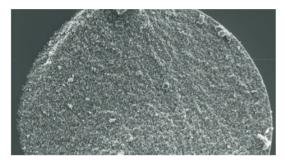
FE-SEM picture of a cut through a Kromasil 300 Å particle at 5 000 x magnification.
