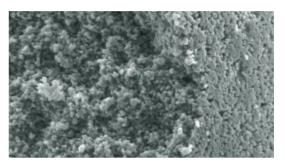
FE-SEM picture of a cut through a Kromasil 300 Å particle at 35 000 x magnification, showing both the outer surface and the fracture through the particle.
