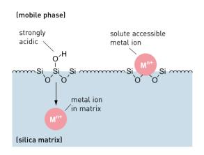
Increased acidity of silanols provides a higher possibility for ion-exchange interactions at any given pH. Moreover, metal ions present in the silica surface layer are able to interact directly with analytes that have Lewis-base properties.
