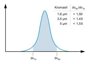
A narrow particle size distribution allows the user to avoid high backpressure due to low bed porosity. To define and secure a narrow particle size distribution, all Kromasil products have to pass stringent quality control specifications of  $dv_{90}/dv_{10}$  ratio. This specification is quite demanding on the manufacturing process, and provides a superior product compared to others in the marketplace today which only have a specification of  $dv_{90}/dv_{10}$ .
