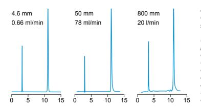
All Kromasil pre-packed columns are delivered with a minimum performance guarantee of at least 40 000 pl/m for 10 µm particles. For larger diameters DAC columns are recommended. The performance obtained in analytical columns can be maintained all the way up to very large industrial scale DAC columns, and in the example an 80 cm ID DAC column is proven to show analytical performance. The scale-up factor from the analytical column in this case is 30 000 times.
