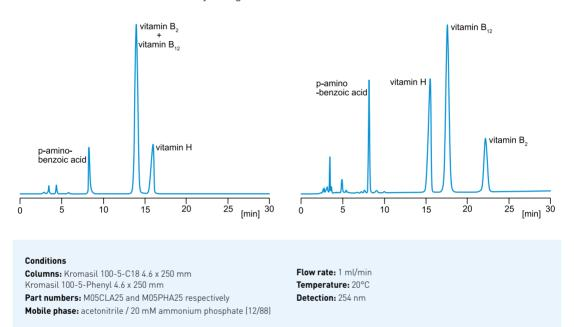
In cases where there is a need to use a completely wettable phase, or when the compounds in the sample have aromatic structures requiring unique selectivity for n-n interactions between the phenyl bonded phase and the solute, Kromasil Phenyl phase can be used. Kromasil Phenyl is derivatized using a mono-functional silane, followed by an extensive endcapping. The result is a stationary phase with high stability, high reproducibility, and symmetrical peaks for basic compounds.
