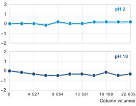
Conditions Column: Kromasil 100-5-C18 3.0 x 50 mm Part number: M05CLC05 Mobile phase pH 2: acetonitrile / water / triflouroacetic acid (TFA) (50/50/0.1) Mobile phase pH 10: acetonitrile / water / triethyl amine [TEA] (50/50/0.25) Flow rate: 1.0 ml/min. Temperature: 20°C Column volumes: 22 635
