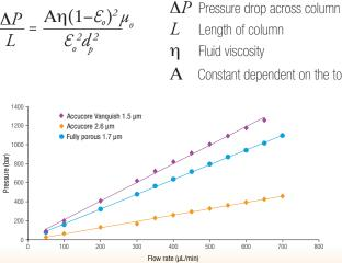
Porosity of the packed bed E Superficial velocity μ Particle diameter
