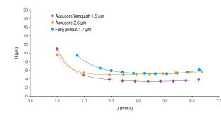
Accucore Vanguish UHPLC columns are more efficient at optimum flow than sub-2 µm fully porous and 2.6 µm solid core columns. Efficiency is maintained over a wider linear velocity range.
