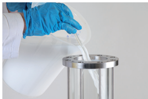
FIGURE 8 Pouring the resin
